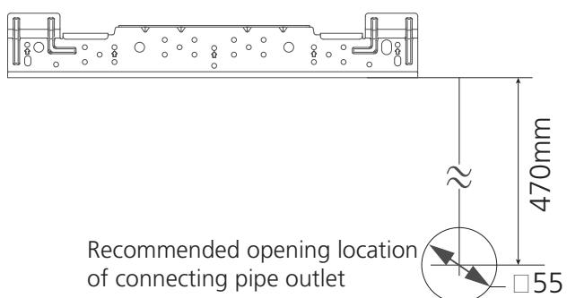
Drainage pipe fixing requirements
